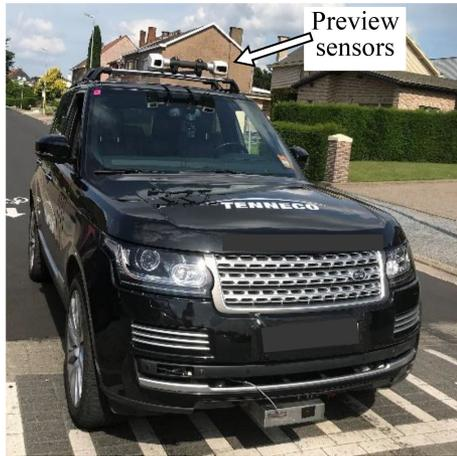
Fig. 2. ACOCAR vehicle demonstrator with preview sensor.
