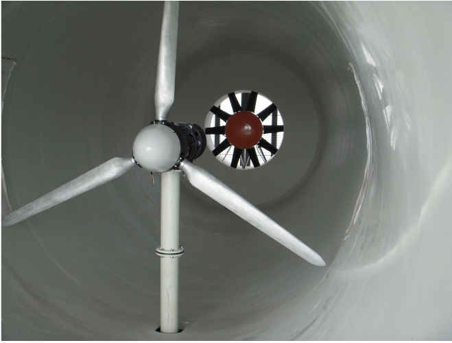
Fig. 2. The laboratory wind turbine set-up.
