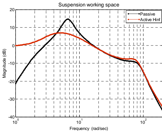
Fig. 8. Bode plot of the normalized suspension deflection – Reliability criterion
