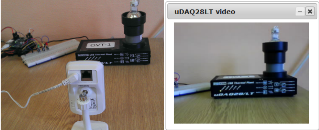
Figure 5.9: Wireless IP camera used in ArPi Lab (left) and its image displayed in GUI (right)
